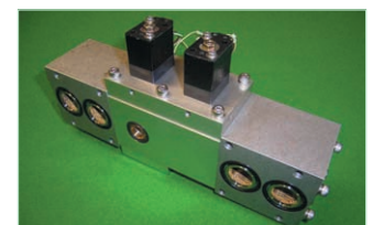
Figure 5. Energy saving anti-skid valve
